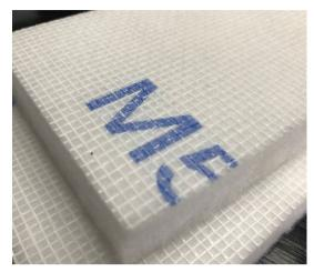
A560G offers fine filtration grade of M5 to EN779 / ePM10 50% to ISO16890, making it suitable for filtering air entering a spray booth above a vehicle through the ceiling in a down draught spray booth.
