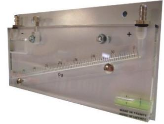
Red liquid within the inclined manometer will clearly and accurately indicate the differential pressure across bag and panel filter sections, and also pressurised rooms, clean rooms and ventilation networks.
