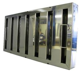
The Baffle Type Grease Filter's smooth surface enables deposited grease to run off via the drainage holes, to grease collecting trays in the canopy or grease filter housing, where it can be easily disposed of. Efficient grease removal by Baffle Type Grease Filters minimises grease build-up in the kitchen extract ductwork system and ensures that duct cleaning requirements are kept to a minimum.
