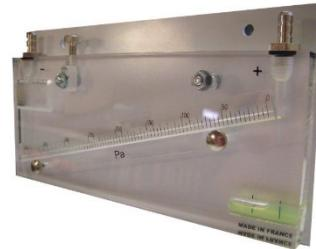
Red liquid within the inclined manometer will clearly and accurately indicate the differential pressure across bag and panel filter sections, and also pressurised rooms, clean rooms and ventilation networks.
