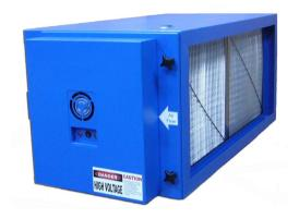
A single pass ESP will achieve a grease and smoke removal efficiency of 95%. Where efficiency is critical (eg. Low level kitchen extract) a double pass ESP is recommended to achieve a 99% efficiency.
