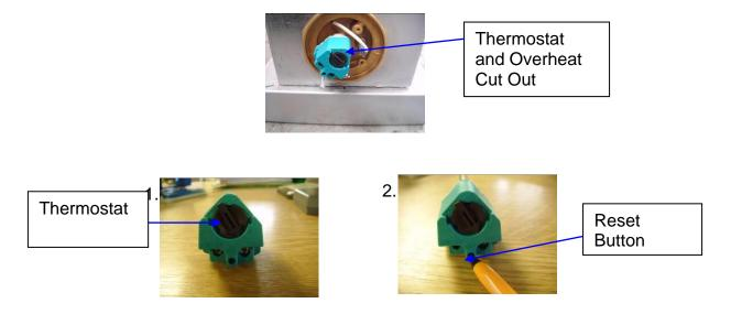
The black arrow with the dial is used to adjust the temperature of the cleaning tank (picture 1), moving the dial toward the + sign to increase the temperature and move it to the – to reduce the temperature. In the event that the heating element overheats a safety cut out will be initialized.
