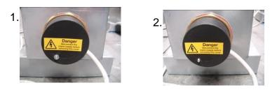
The reset switch and thermostat for adjusting the temperature of the cleaning tank are situated inside the black plastic safety cover on the back of the cleaning tank's heating element (picture 1). Release the small nut which holds the cover in place using a suitable tool (picture 2) and remove the black safety case.
